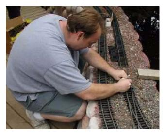
We did not expect cutting and bending stainless steel rail to be so difficult. Dave Linn brought an air grinder to cut rail. It was still a lot of work. Jeff brought a rail bender, but Gary preferred the handle on our rail bender. I also observed Jeff bend an assembly of rail across his belly. He commented that brass rail was easier to bend.
