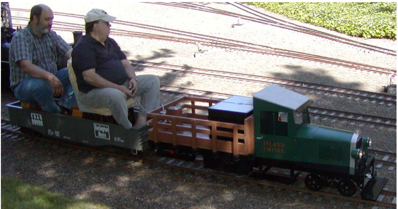
One of Tom's associates built this great model of the "Goose #1". It is battery powered and uses two wheelchair motors connected to the drive axles.
