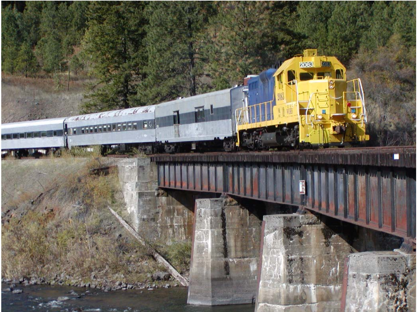
An opportunity for a run-by across the bridge where the Wallowa and Grande Ronde Rivers meet. The car behind the locomotive has been converted to a power car to supply heat and power to the passenger cars.
